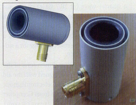
4. A CAE model of the feed (a) is shown alongside the actual fabricated feed (b).
