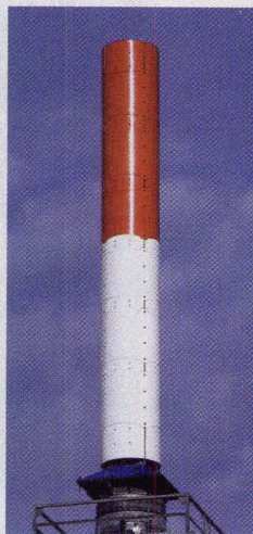
1. A small cross section and cylindrical radome design helps dramatically reduce the wind loading on these broadcast antennas. [Photo courtesy of Radio Frequency Systems (RFS; www.rfsworld.com ).]
