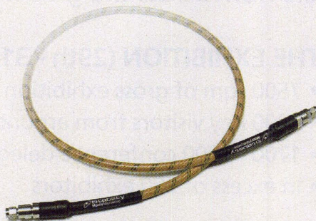
1. Stability RF/microwave cable assemblies can be ordered in standard lengths of 24, 36, 48, and 60 in. for use to 26.5 GHz and to 40 GHz.
