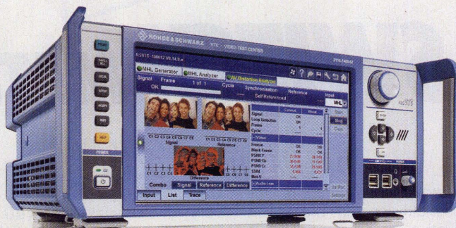
This newly developed video test center can test both the functionality and compliance of digital video interfaces, which are found in products ranging from set-top boxes to tablet PCs and smartphones.
